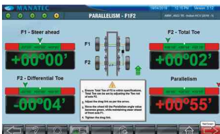
Alignment of Front twin steerable axles to maintain parallel condition
